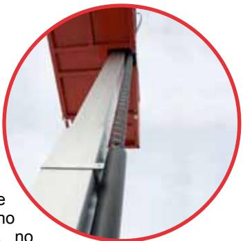
The revolutionary mast lifting system designed by BRAVI PLATFORMS for all its platforms models represent a real change on its sector! The mast made of a special extruded aluminium is 100% maintenance free! No more chains to be regularly inspected, no more grease or lubricant required, no maintenance: a real low cost ownership!
